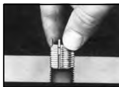
3. Screw in insert until slightly below surface. "Kees" act as depth stop.
