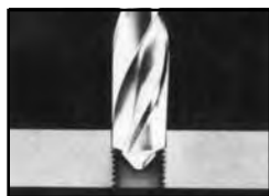
1. Drill out old threads, using standard drill.
