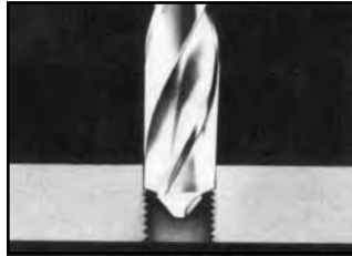
1. Drill out old threads, using standard drill.
