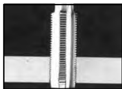
2. Tap new threads, using standard tap.
