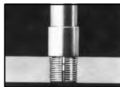
4. Drive "Kees" down with several light taps on installation tool.
